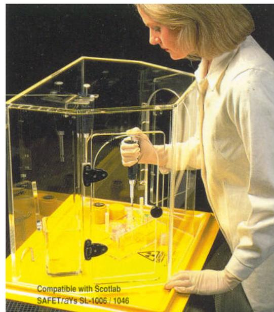
**Figure 2** Workstation comprising a beta cab and drip tray
