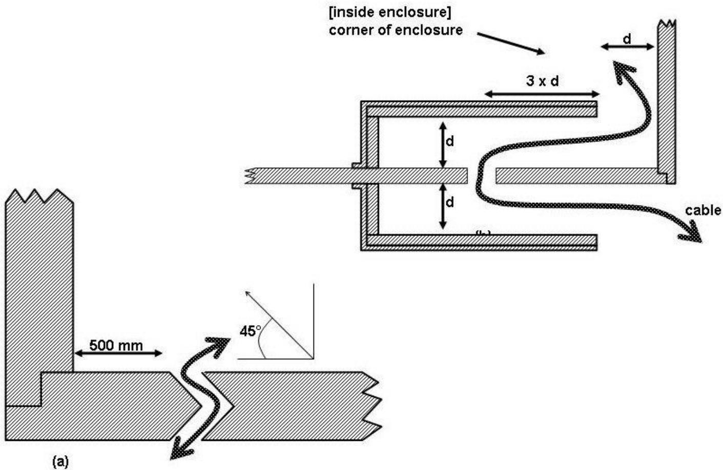
Shielded cable entry points; a - simple chevron facing the corner of the enclosure, b - box design
